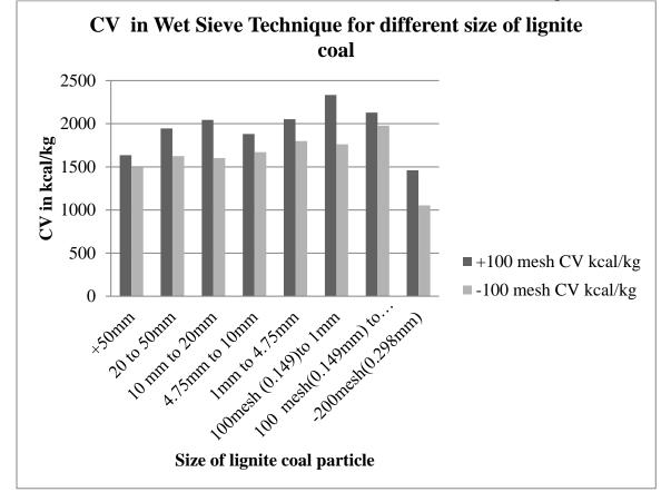
Fig. 4 The representation of CV kcal/kg in wet sieve Technique for +100 mesh size and -100 mesh fine size 0.298 mm to 50 mm
