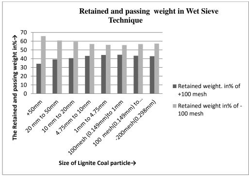
Fig. 1 The representation of retained and passing weight in wet sieve technique for +100 mesh and -100 mesh size
