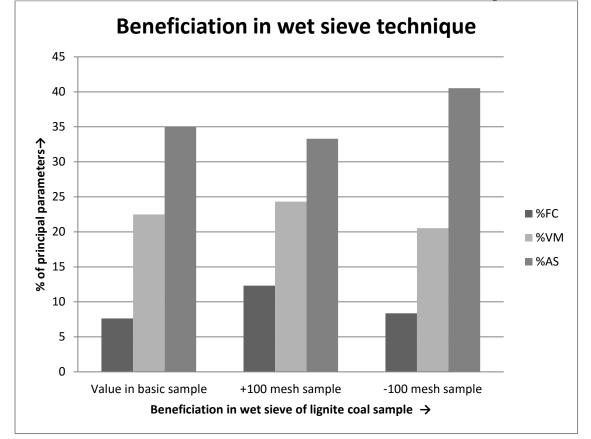
Fig. 3 The representation of beneficiation in wet sieve Technique for +100 mesh size and -100 meshes rang in 0.298mm to 55 mm.
